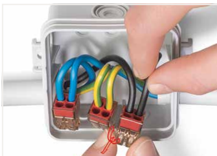
Removal: Hold conductor to be removed and twist alternately left and right while pulling the connector.
