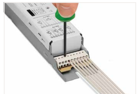
Removing a conductor via 1.0 mm Ø 206-841 Disconnection Tool.
