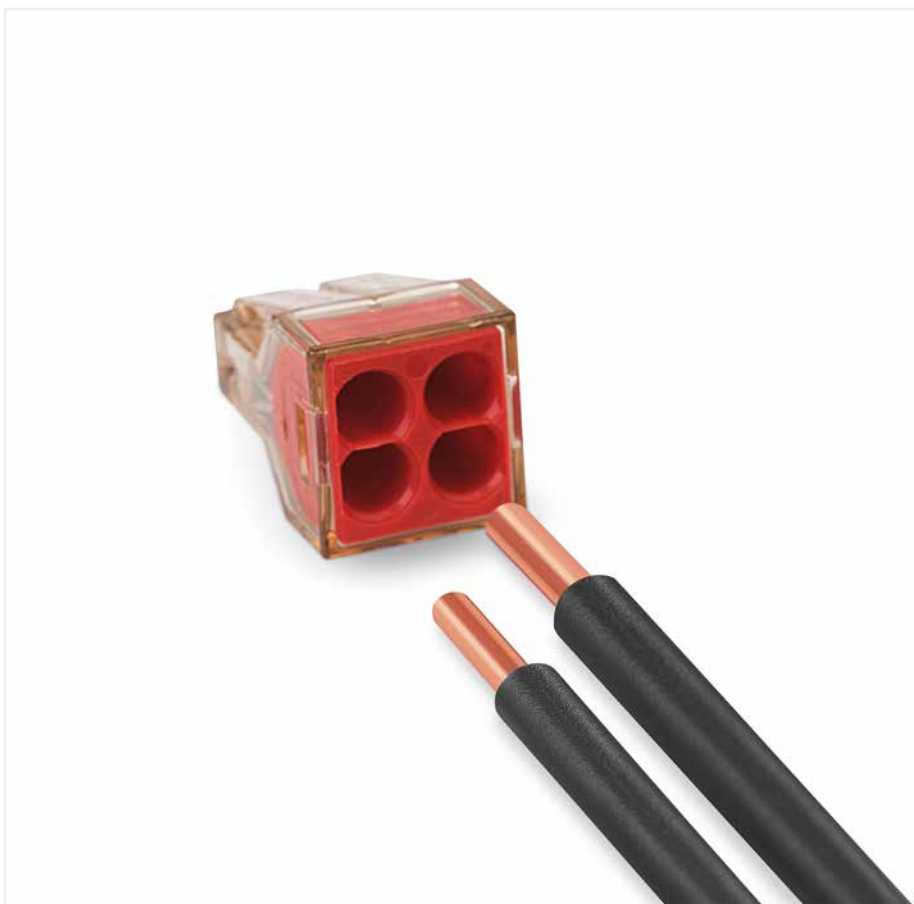
Removal: Hold conductor to be removed and twist alternately left and right while pulling the connector.
