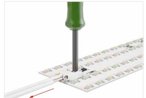
Inserting/removing fine-stranded conductors by lightly pressing on a push-button (e.g. via 206-861 Operating Tool).
